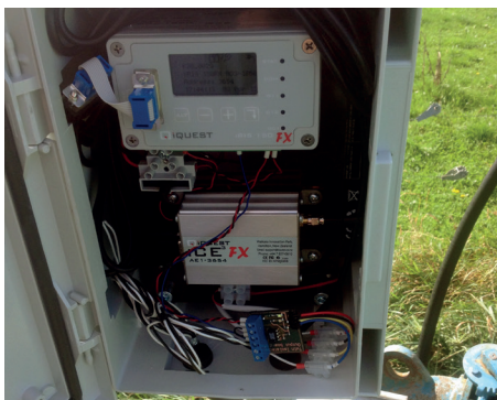
iRIS 150FX mounted in an iBox custom enclosure
