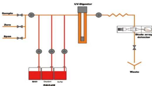
Digested sample flow to measuring cell and measured By spectro-photometrically.
