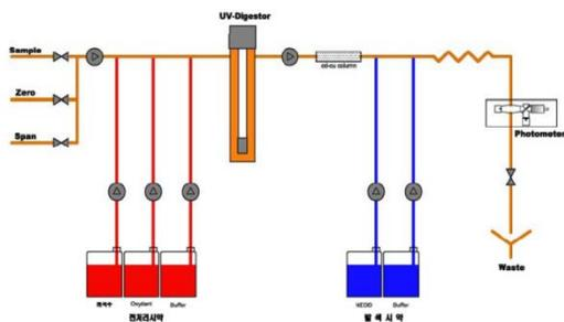
Digested sample flow to reduction column(or reagent) to change as nitrite and colored by NEDD and measured by photometrically.
